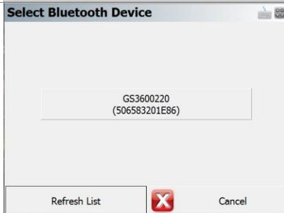
Select the bluetooth modem associated with the GS18. The modem will be listed as GS+serial # e.g GS36000220. The serial number is found on the model tag on the bottom of the GS18.
