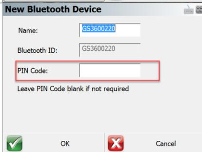
There is no PIN code needed for the GS18. Leave this field blank and select the OK button.
