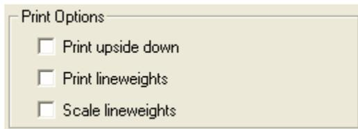
Prints upside-down: Some plotters require this to be set to orient the drawing on the paper correctly.
