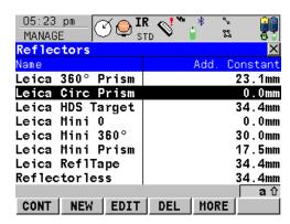
Example: Let's assume you are using a Leica 360° Prism for your foresight shots, and have Leica Circular Prism setup on a tripod at your backsight. In FieldGenius you would define an offset of 23.1 for the foresight, and 0 for the backsight.
