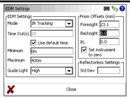
Total Station prism offsets should be handled by FieldGenius.
