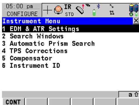
4. On the EDM & ATR Settings Menu, scroll down and check that the ATR Setting is set to Normal. Depending on the conditions you are surveying in you may need to change this from time to time to one of the other ATR modes, but for most applications leaving this set to Normal will be ok.
